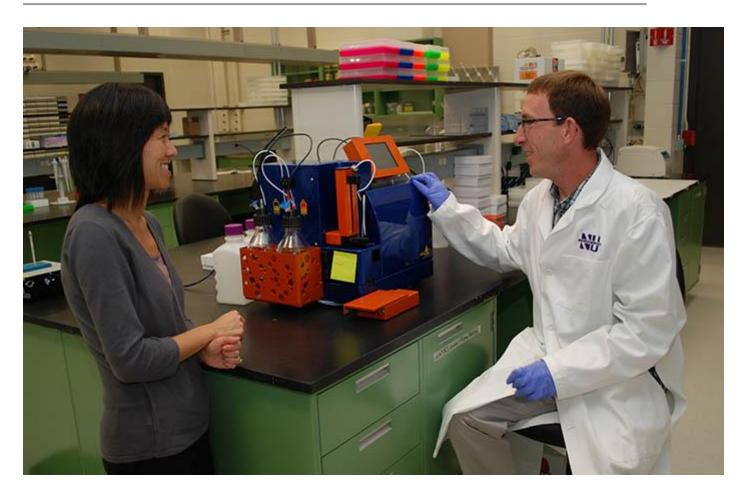
Edith Chen and Greg Miller analyze a blood sample using a cell sorter, which can isolate specific types of cells, in their new research lab.
